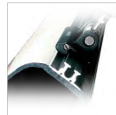
Luff groove tracks for sail flexibility
