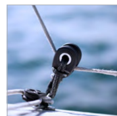
Cheek plates rotate to open block
