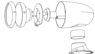
SPARE PARTS: ME000FR010 QUICK EXTENSION LEAD 4 MT. 7000002008 BASE MOTOR GROUP 7000002009 BODY MOTOR GROUP SPARE BULBS FOR 7000000012/24 NOW DISCONTINUED 7000001012 SINGLE HEADLIGHT HALOGEN 12VOLT
