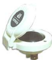
FS200 Foot switch Load capacity:200A Terminals: 8mm Mounting hole: Φ50mm
